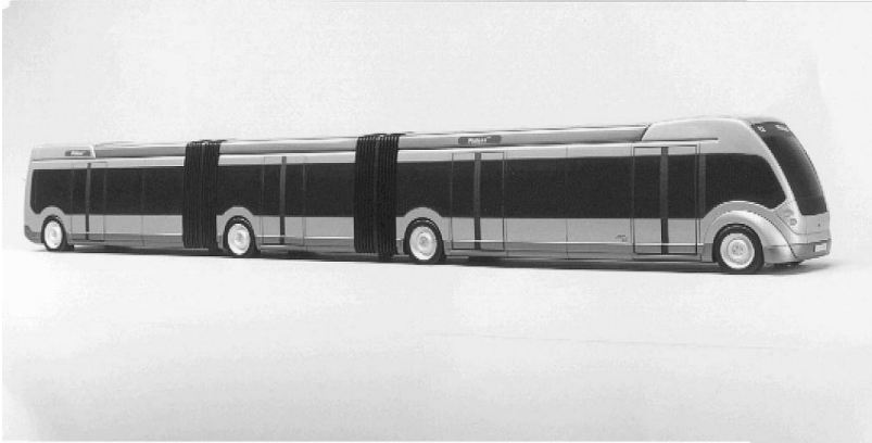
Figure 1.1: Scale model of double articulated vehicle as is going to be used in Eindhoven
