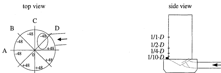
Figure 5.4 :: Definition of measuring positions for the in-cylinder LDV experiments on the steady-flow rig
