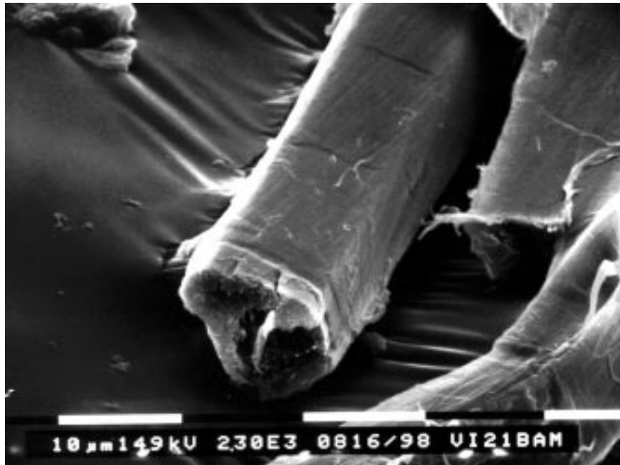
Figure 7. Dry Duralin single flax fibre.
