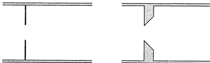
Figure 5.17: The two diaphragms that were studied numerically. On the left is the thin diaphragm, which is an approximation of a line diaphragm, and on the right is a two-dimensional representation of the actual diaphragm used in experiments.
