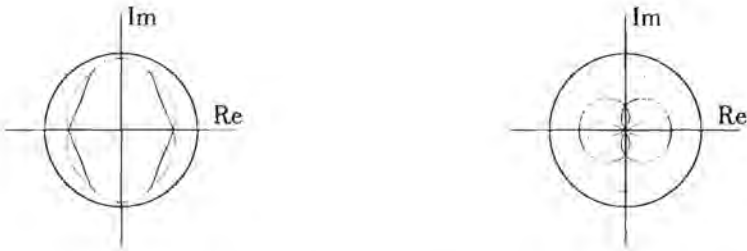
Figure 4.12: Root-maps of a second-order two-dimensional recursive system.
