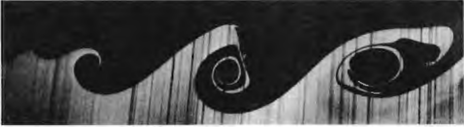
Figure 6.2: Parametric resonance in an unsteady Kelvin-Helmholtz flow. The upper stream is perturbed sinusoidally at half of the natural frequency and as a result the motion is locked into the subharmonic. (Copyright © Van Dijke 1982, The parabolic press - Reprinted with permission).
