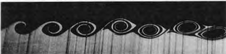
Figure C.2: Development of Kelvin-Helmholtz instability at the interface of two fluids (Copyright © Van Dijke 1982, The parabolic press - Reprinted with permission).
