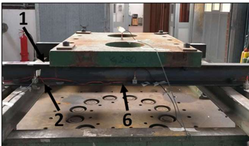
Figure 6.9 Rigid shock test: strain gauges no. 1 (on top faceplate), 2 and 6 (on bottom faceplate) set up
