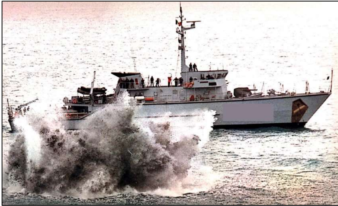
Figure 8.25 Underwater shock test explosion (image taken from [8.18])
