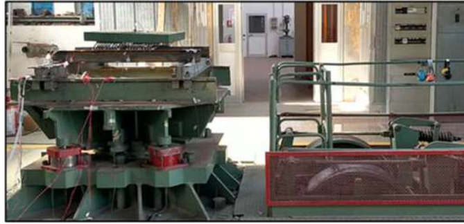
Figure 6.16 Shock test with mountings: effects immediately after the drop hammer (image taken from recorded video)
