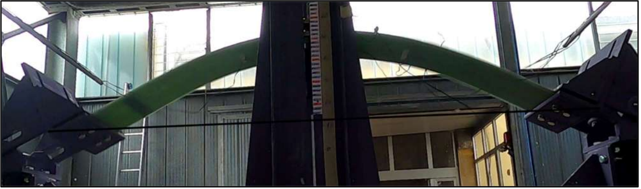
Figure 7.13 Impact no. 6 - Maximum deflection (420 mm) for G1 g/m 2 , 20 mm, manufacturer "D" specimen (image taken from a recorded video)
