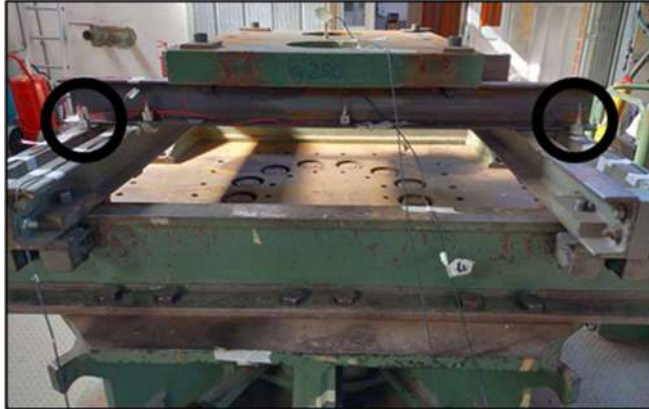
Figure 6.7 Rigid shock test: accelerometers setting. Accelerometers on supporting channels are circled
