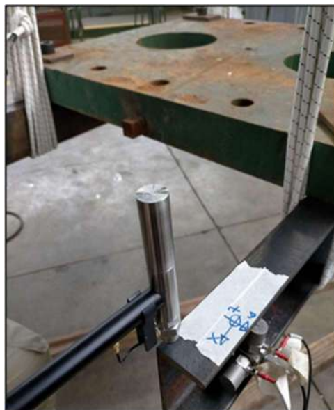
Figure 6.3 Experimental modal analysis: vertical hammer and accelerometers in point no. 1
