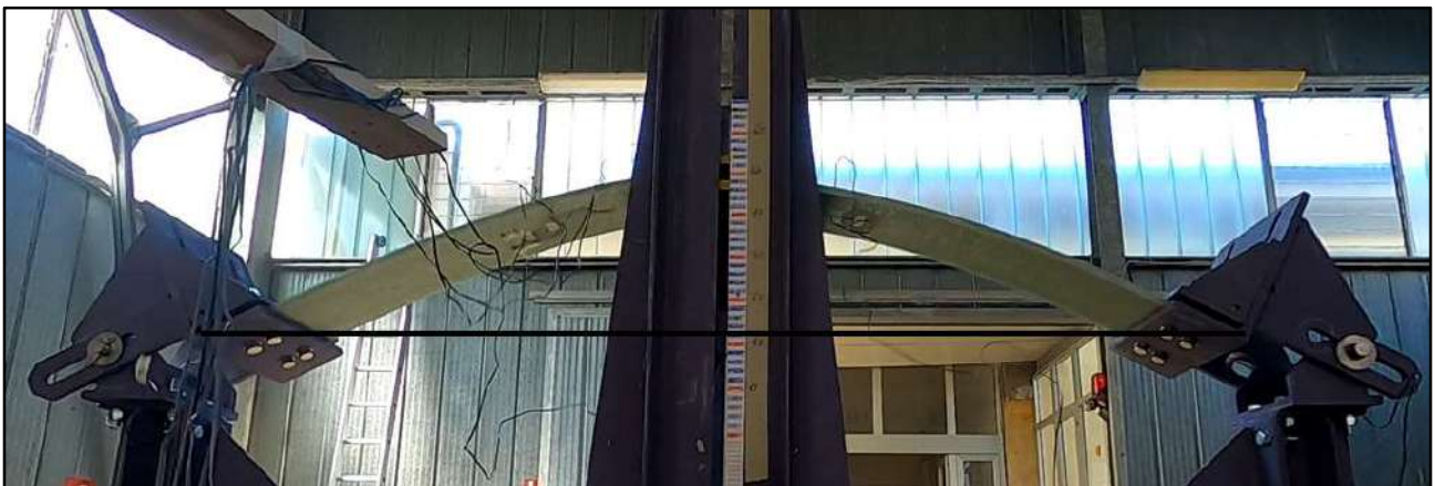
Figure 7.12 Impact no. 6 - Maximum deflection (380 mm) for G2 \text{ g/m}^2 , 20 mm, manufacturer "D" specimen (image taken from a recorded video)
