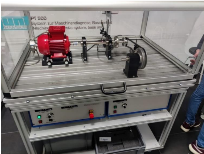
Fig. 1. PT-500 tool for vibration analysis training
