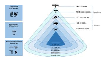
Fig. 3: NTN platform types and architecture options.
