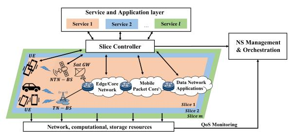
Fig. 5: NS high-level architecture.
