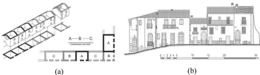
Fig. 1 Aggregate buildings: a evolution by the individuation of different SUs (adapted from Giuffrè 1990); b geometrical survey of buildings in aggregates
