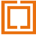
Figure 1. Geometrical structure of a split-ring resonator (SRR) unit-cell.
