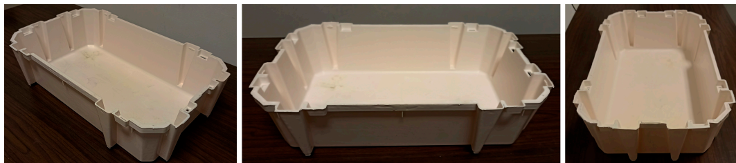
Figure 1. Injection-molded tray. All the specimens utilized for mechanical and biodegradation tests were obtained from the flat areas of the sides of the tray.
