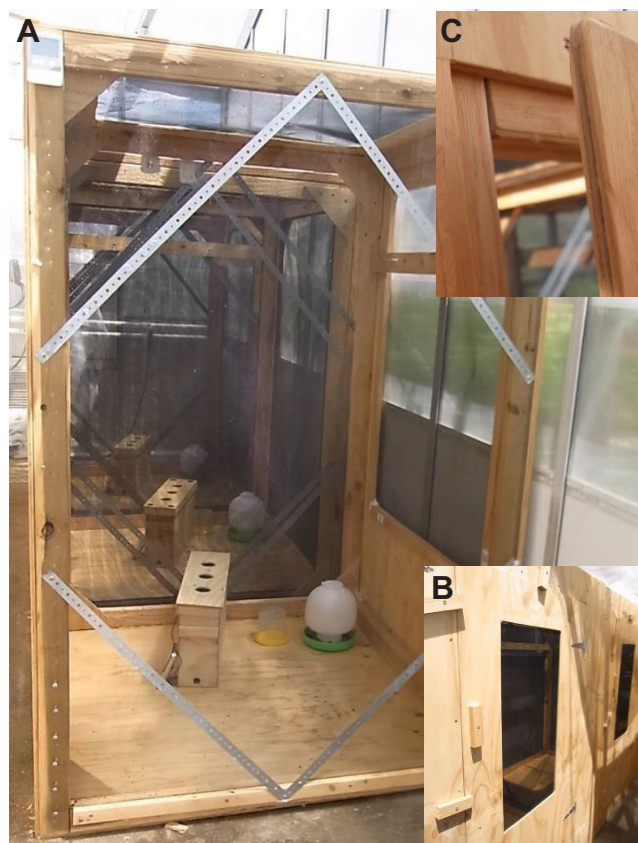
Fig. 1. The cage system. (A) The system includes a hive box and feeders (door not visible but located on the left side of the cage). (B) External view of the secure timber door with insect screen panel and closure toggles. (C) View of the overlapping cage door panels for secure fit with the cage frame. The cage system was developed and used to successfully house honey bee colonies for effect studies. See Materials and Methods, 'Cage design and cost' for specifications of system components.
