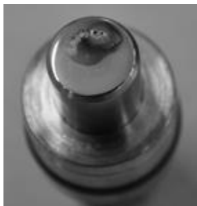
Figure 3.12| Small depressions in Tungsten target caused by high energy electron beam causes ‘pitting’ or small depressions in the target surface. This degradation produces a lower intensity X-ray beam.
