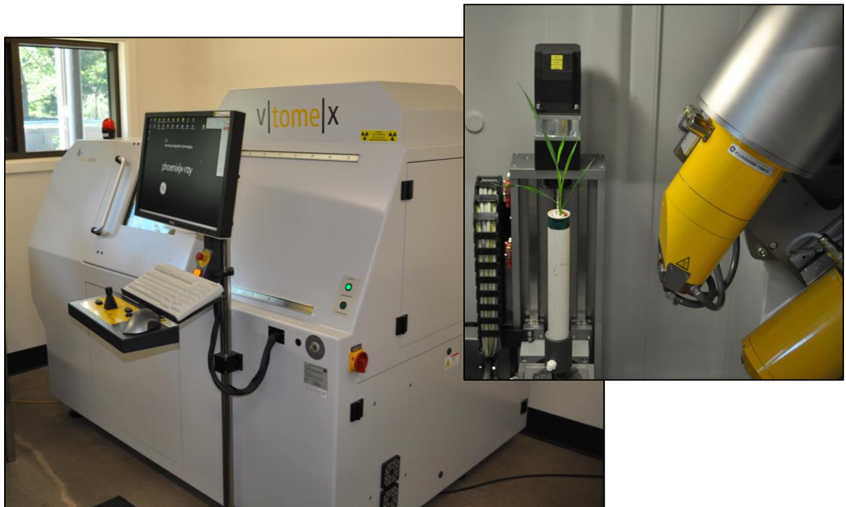
Figure 3.1| (Left) The University of New England V|tomex|s Micro CT cabinet manufactured in 2010 by General Electric Phoenix. (Right) The V|tomex|s interchangeable X-ray sources (pictured in yellow) with the ‘direct’ tube in position (top most tube) picture captured during a scan of 28 day old wheal plant in white PVC tube, mounted in grey PVC mounting on the CNC manipulator.
