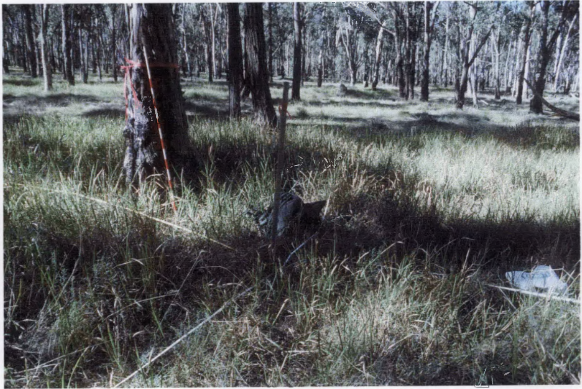
Figure 4.1. Centre of the site (steel marking post) with four tapes running along the compass axes setting out site layout, in an HSS Tablelands site.
