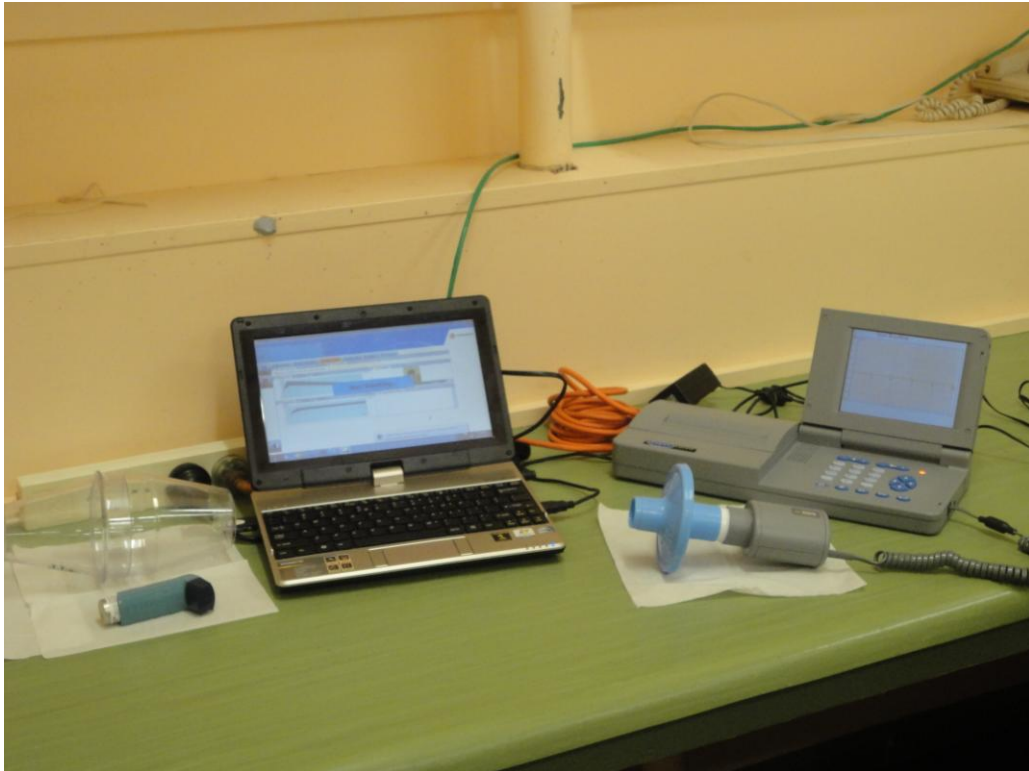
Figure 2.2 – Experimental set up showing the Super Spiro spirometer with microbial filter attached to the flow sensor, personal computer, Ventolin and a spacer device.
