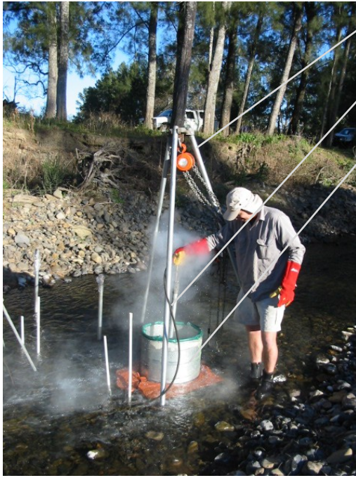
Plate 2.8 Freeze-coring at the downstream log sill at WUM on the Williams River. The stilling dam is the cylindrical metal object at the base of the tripod. A plastic flange at the base of the stilling well prevents near-bed flow from dissipating the effects of the freezing. Stream flow is from right to left.
