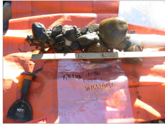
Plate 2.9 A frozen core from the downwelling zone at the head of the upstream riffle at WUM prior to cutting into 10-cm sections (black lines on the ruler).
