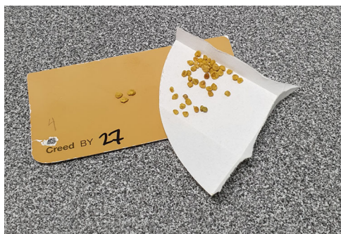
FIGURE A4 Color matching. The three pellets on the paint card were reserved for acetolysis, while the remainder of the pellets were stored in a labeled paper envelope.
