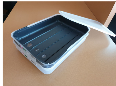
FIGURE A1 Tray for sorting pollen pellets. The top plastic container is lined with adhesive matte black vinyl. The holes in the top container allow pollen to be collected in the bottom container when gently pushed toward the holes with an artist's fan-shaped brush. The lid keeps the pellets secure inside during transport.
