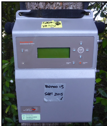
Fig. 2. Wildlife Acoustics Song Meter SM3 audio recording unit in the field.
