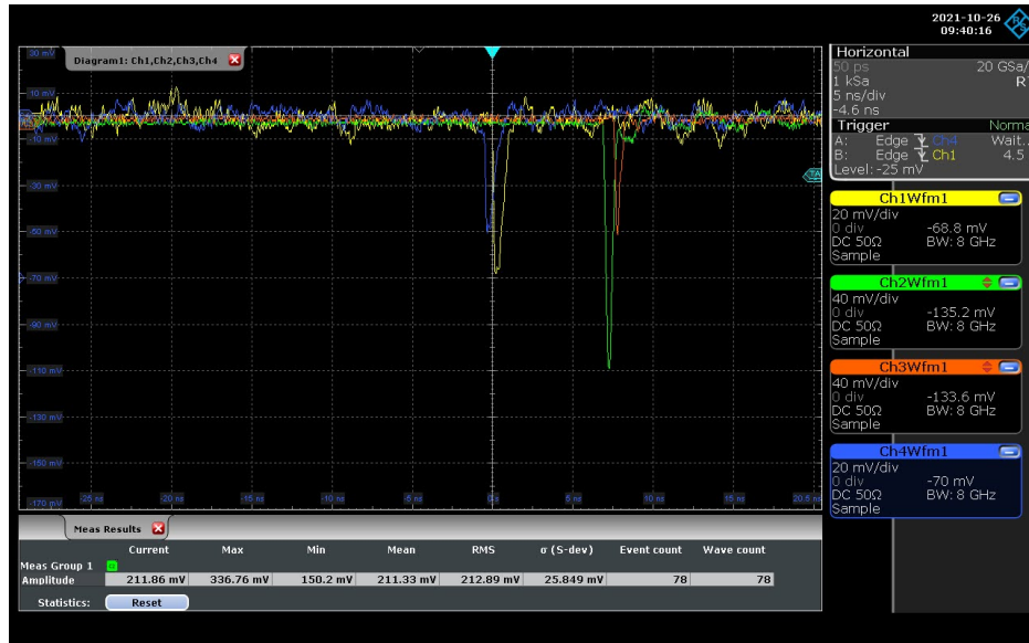
Fig. 5.4 A typical event. The signals from the two silicon sensors are shown in yellow and blue while the signals from the two MCP-PMTs are shown in green and orange. The relative timing between silicon sensors and MCP-PMTs signals is digitally adjusted to optimize the trigger condition.
