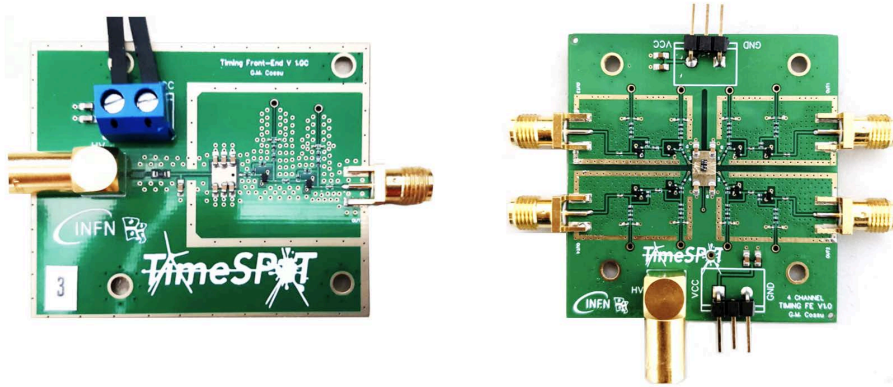
Fig. 5.2 The front-end boards: (left) single-channel and (right) four-channel versions. The sensors are attached with conductive tape to the large metal pad at the board centre and the readout electrodes are wire bonded to the input pad. The large metal pad provides the bias to the sensor under test.
