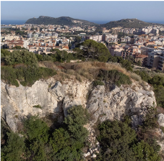
Fig. 7 - Wide view (1) and traces of the fort of Sant'Ignazio identified during the UAVs survey. Among these a portion of the trench that housed the positions for artillery (2), masonry structures (3) and a stretch of a connecting path between different levels occupied by the works (4).
