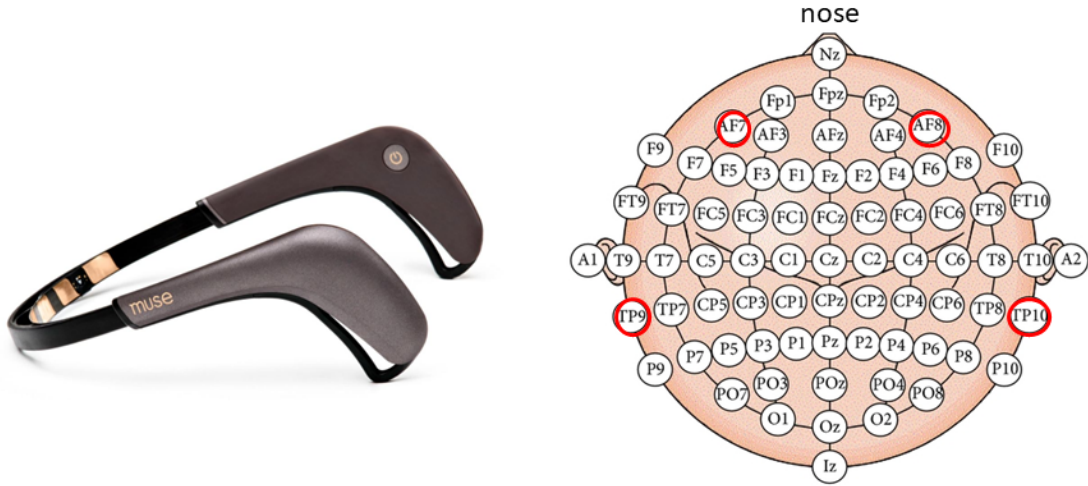
Figure 2.2: On the left, the figure shows the low-cost portable EEG sensor Muse headband version 2 of InteraXon used in the works presented in Chapter 3 and Chapter 4. In red, on the right, we show the position of the Muse’s electrodes on the scalp according to the 10-20 electrode placement system.
