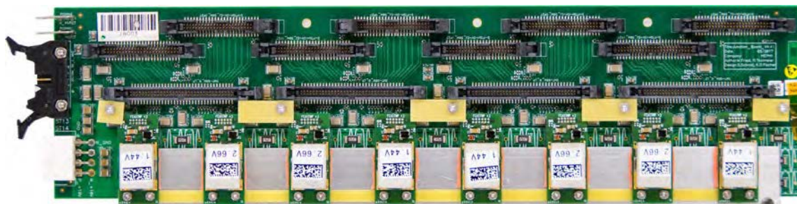
Figure 17. Junction Board with eight DC/DC converter modules.
