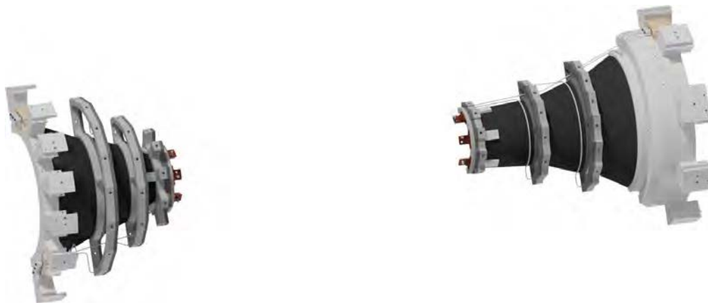
Figure 24. Support structure of the +x half of the SVD, composed of carbon fiber cones, stainless steel end-rings, and aluminum end-flanges. Cooling pipes are interfaced through ceramic isolators (in beige plastic holders) at the end-flanges. The BWD (left) and FWD (right) parts are later connected by the outer-cover (not shown).
