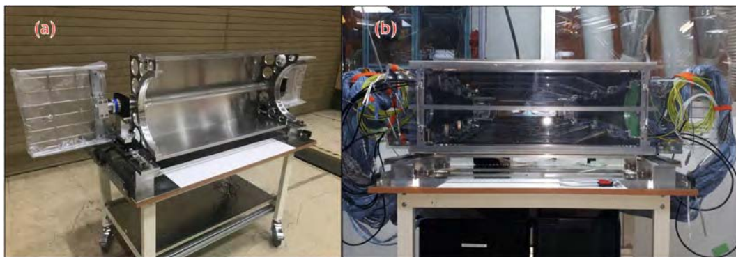
Figure 67. (a) The bare SVD pick-up tool on the storage table. (b) SVD half-shell on the storage table held by the pick-up tool, with the front cover installed.
