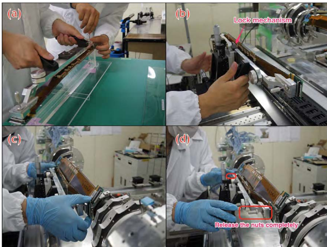
Figure 63. Key steps of the ladder mount procedure. (a) the ladder mount tool is attached on the ladder using the fixing screws and the nuts; (b) the ladder mount tool is fixed on the ladder mount stage; (c) after the alignment of kokeshi-pin heads with the corresponding holes, the ladder is inserted in the end-rings; (d) the ladder is released from the ladder mount tool. Note that in the actual ladder mount procedures gloves were worn at all times to avoid sensor contamination. Some pictures were taken in early stages of the procedures development, with mechanical samples that required less attention.
