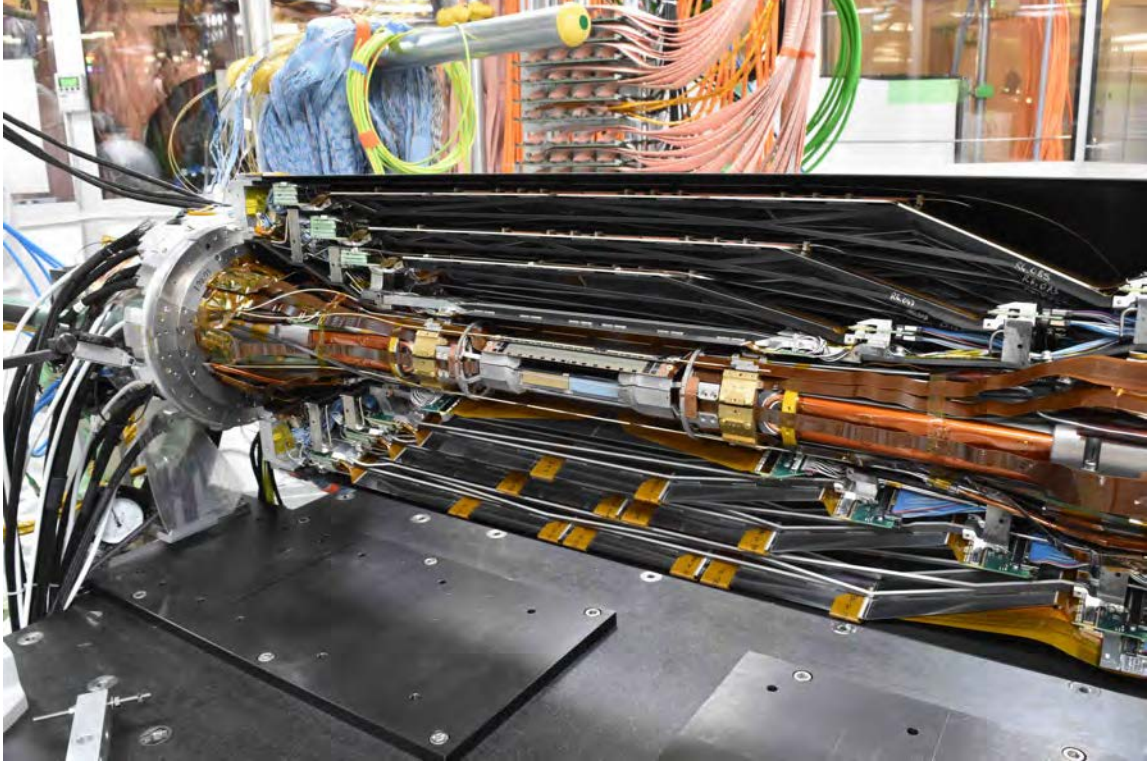
Figure 92. A picture of the first SVD half already coupled to the PXD.
