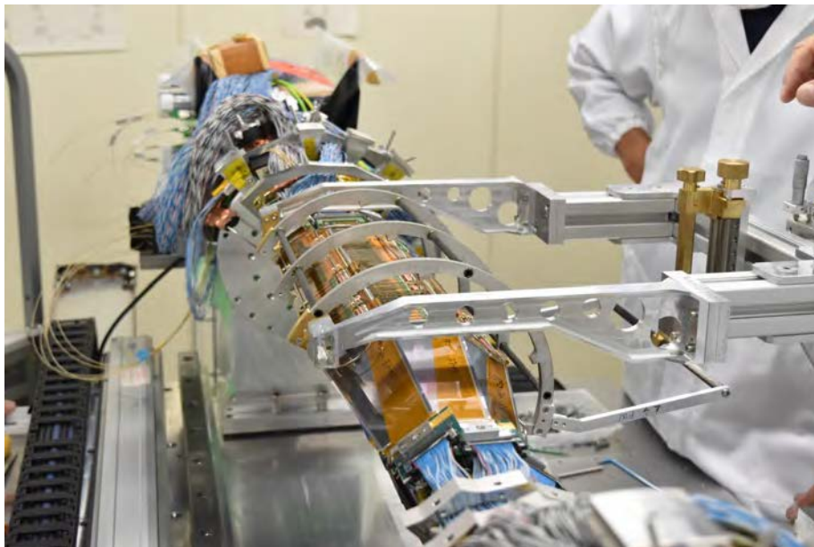
Figure 65. Layer 4 cooling pipe attachment: after positioning the cradle on the Layer 4 half-shell, the pipe is inserted into the CO 2 clamps of the ladders.
