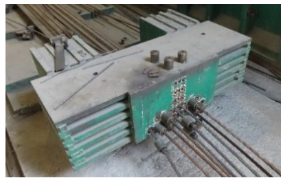
Figure 3-18: Terminal head for strand anchoring.
