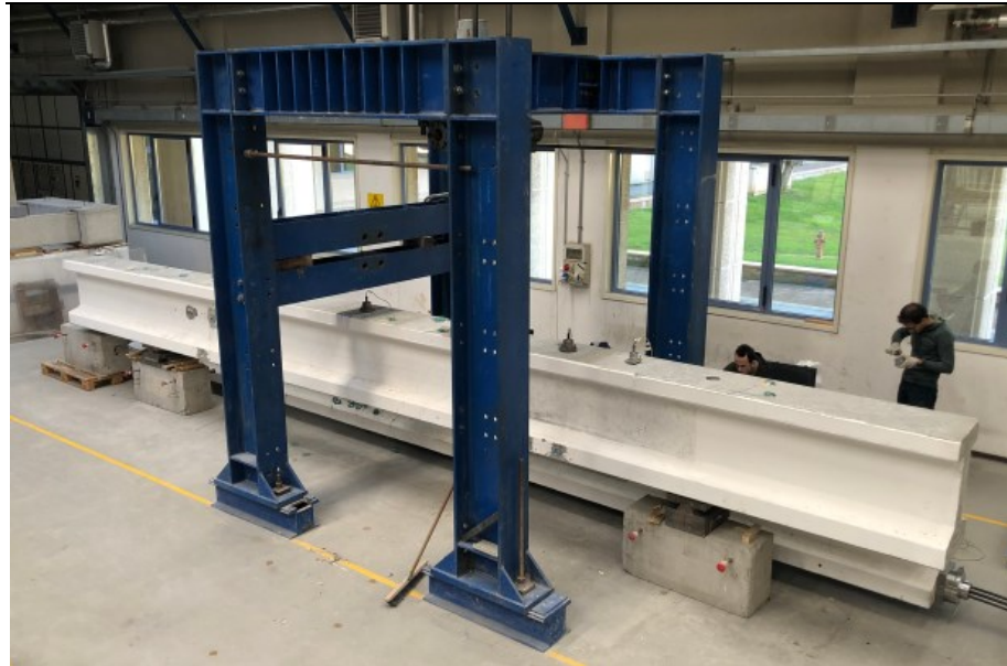
Figure 4-135: Dynamic characterization of beam-A through OMA technique: Picture of the experimental set-up.
