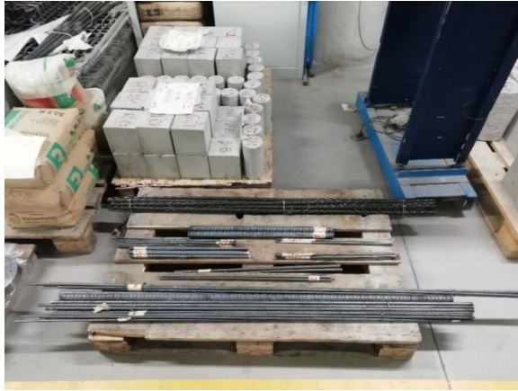
Figure 3-44: Specimens from the casting of the 4 beams and sections of the reinforcing bars.
