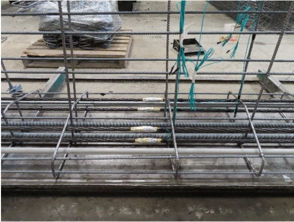
Figure 3-31: Strain gauges below the point of load.
