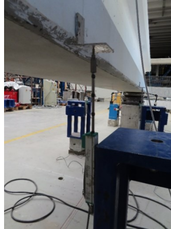
Figure 3-42: Potentiometer in the symmetrical position of the load point.
