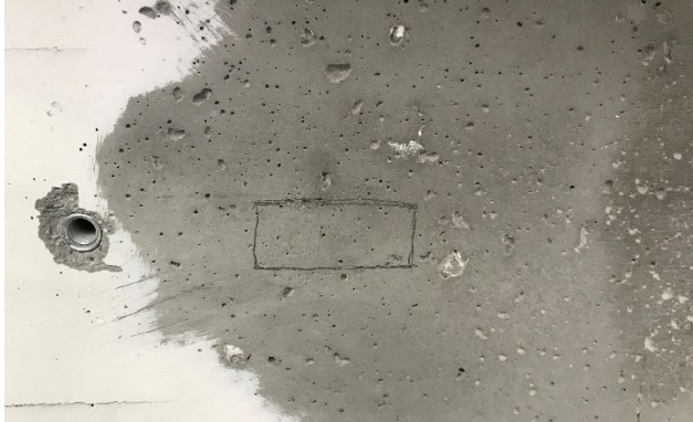
Figure 4-70: Identification of the surface of test SCw_10_GC_6_3 for gluing.
