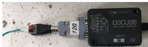
Figure 4-23: Single-channel control unit for the acquisition of strain gauges.
