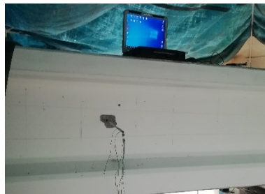
Figure 4-20: The opposite side of the core with cable routing through the web and acquisition hardware.
