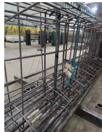
Figure 3-29: Strain gauges at support.
