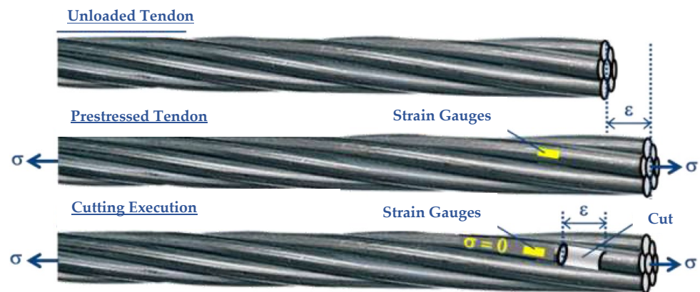
Figure 2-5: Test of cutting a wire of a strand [ANAS S.p.A., 2020] adjust.
