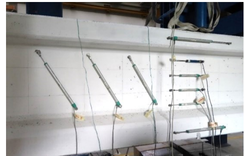
Figure 3-40: Arrangement of instruments in post-tensioned Beams C on face side flanges and web.
