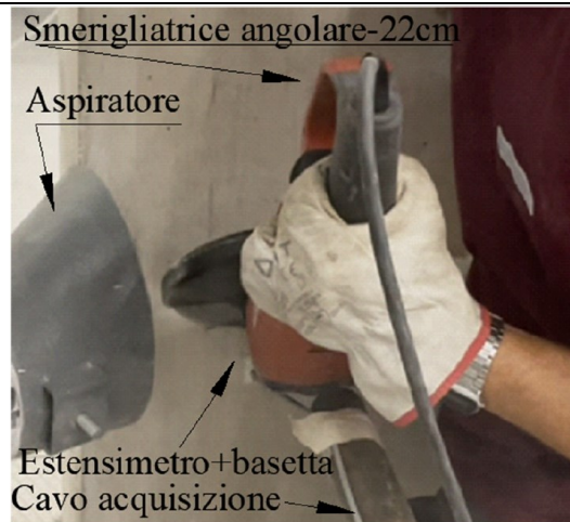
Figure 2-35: Cutting with an angle grinder on one side of the square mesh [Romano and Mazzotti, 2022].
