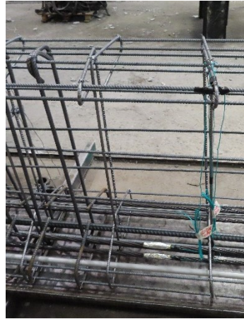
Figure 3-32: Strain gauges at support.
