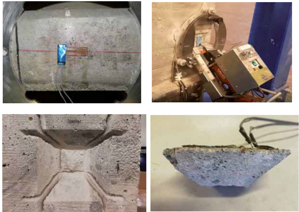
Figure 2-33: Test execution phases with blunt pyramidal specimen [Martinello, 2021].
