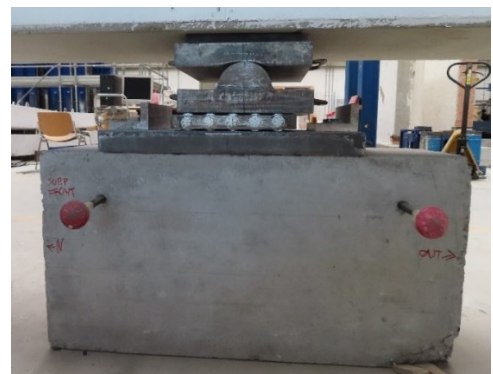
Figure 3-52: Roller support – P side.
