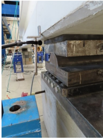
Figure 3-41: LVDT near the simple support (roller)
