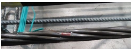
Figure 3-25: Strain Gauge on a wire of a strand.
