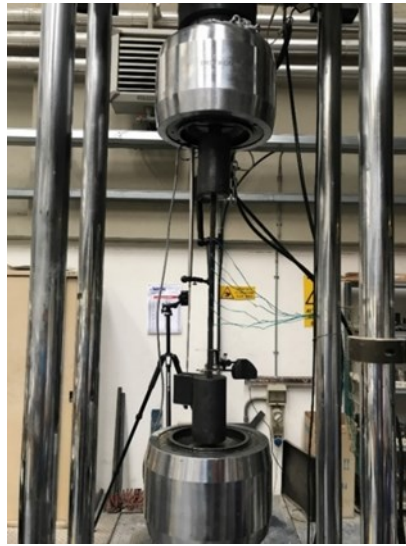
Figure 3-35: Test to verify the differences in the reading of the strain gauges.
