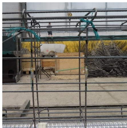
Figure 3-26: Strain gauges with protection on the stirrups.
