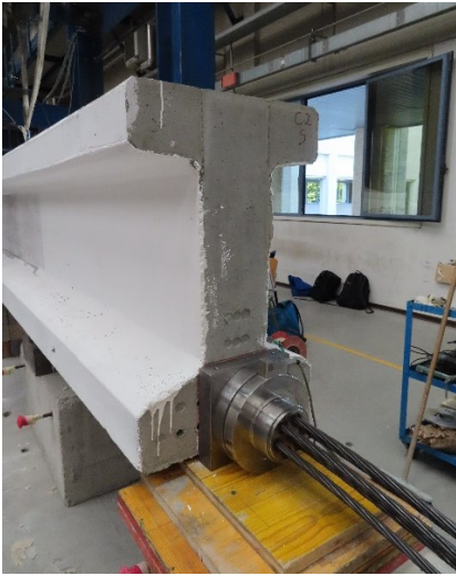
Figure 3-55: Passive beam head.
