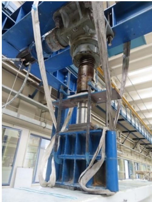
Figure 3-50: Loading system composed of an electromechanical jack load cell and steel thicknesses.
