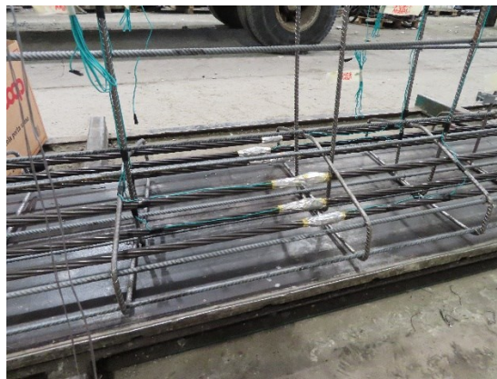
Figure 3-28: Strain gauges below the point of load.
