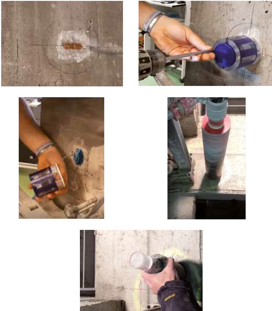
Figure 2-20: Executive sequence of the Instrumented Core [Martinello, 2021].
