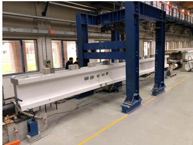
Figure 4-15: Beam C2 with part of additional distributed mass: experimental set-up for the "hammer tests" at N=1126 \text{ kN} .
