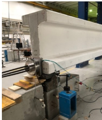
Figure 4-11: Passive header restraint – S-side.
