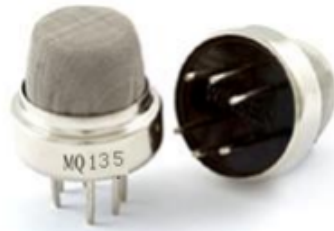
Figure 3.3: MQ135 Semiconductor Sensor for Air Quality. Source: Winsen [121], 2022.
