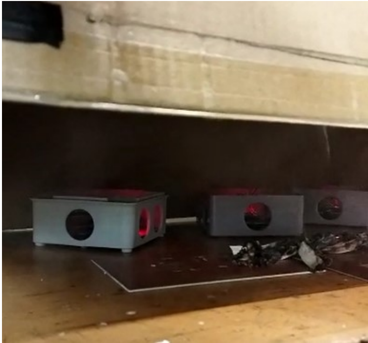
Figure 5.11: Simulation of high gas level with burned paper.
