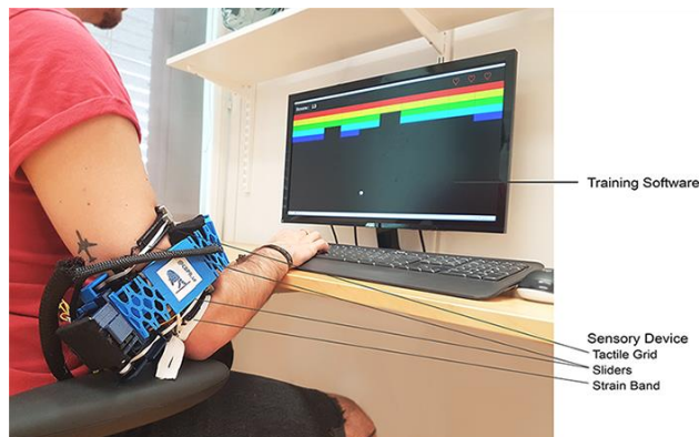
Fig. 5. Wearable somatosensory device for training tactile sensitivity.
