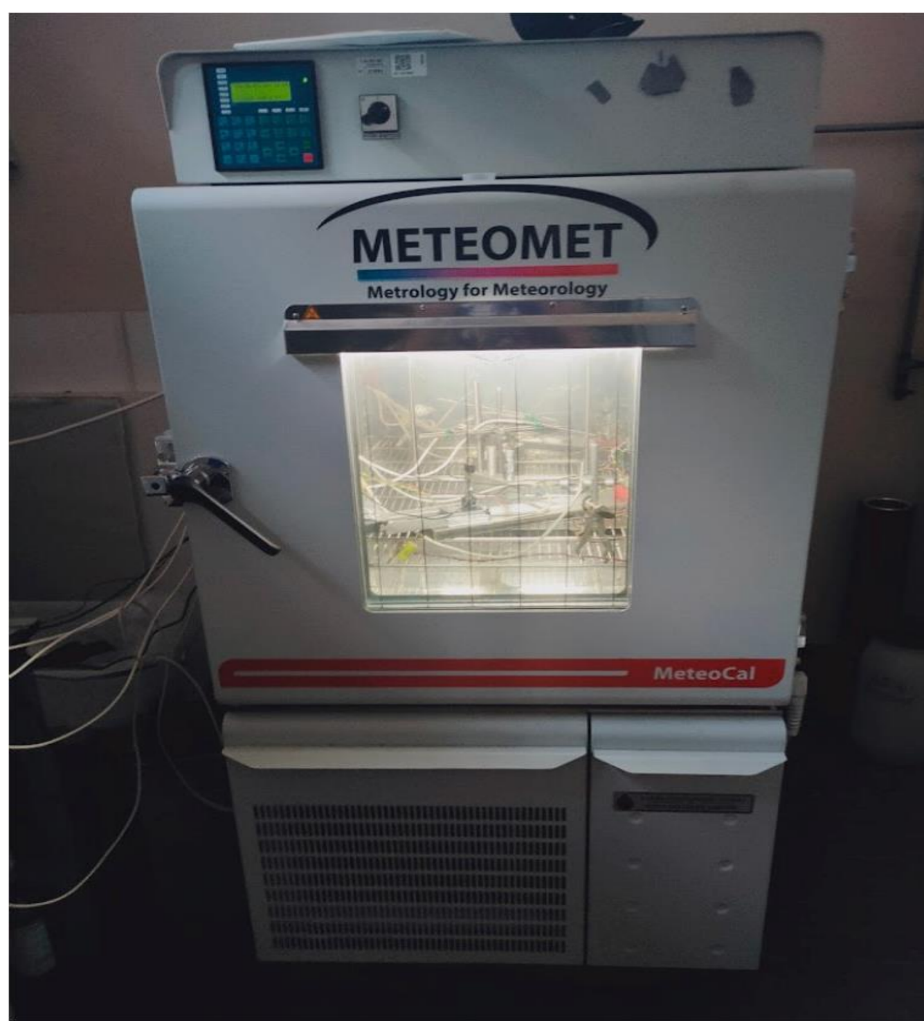
Climatic chamber Kambic MeteoCal KK-105 in operation at INRiM.
