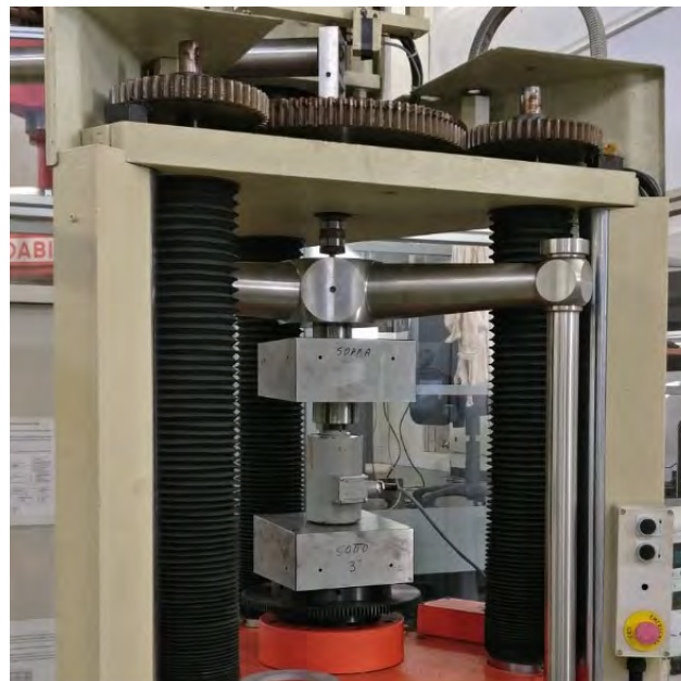
Figure 16 The 20 kN transducer placed between the 3° tilted plates integrated into the MCF30 FSM
