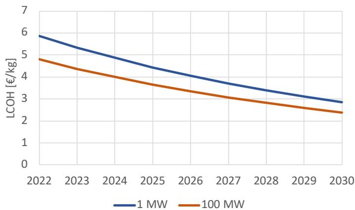
Figure 46: Levelized cost of hydrogen production via electrolysis from solar PV electricity in Spain. Comparison between a small-scale (1 MW<sub>el</sub>) and a large-scale (100 MW<sub>el</sub>) plant.
