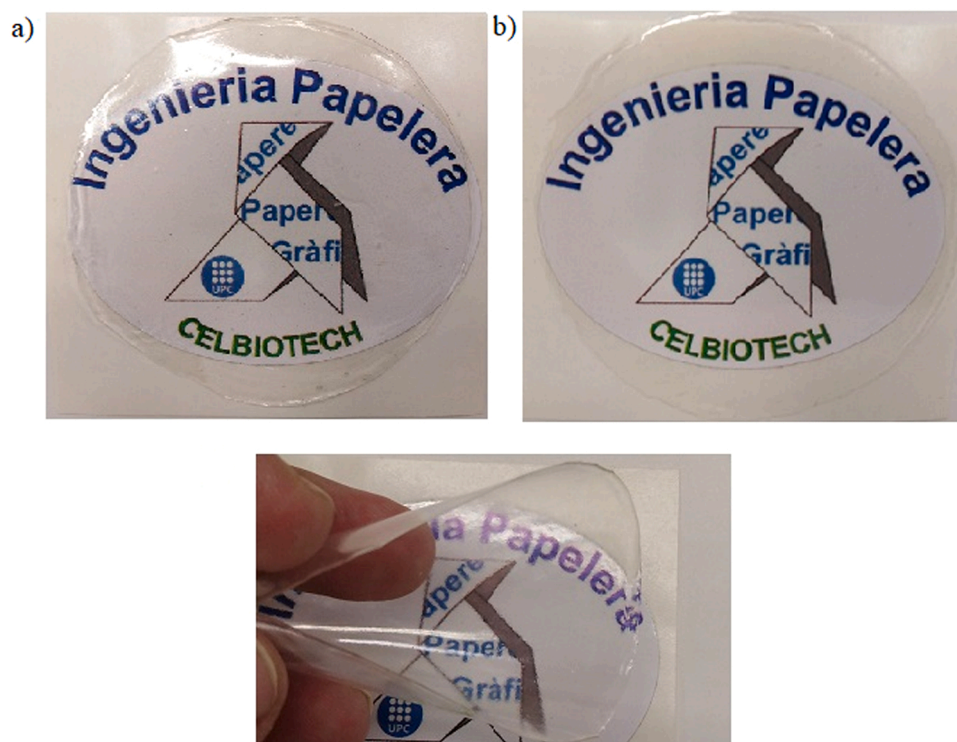
Fig. 11. Visual appearance, qualitative transparency and flexibility of cellulose-grafted PCL nanocomposite films containing (a) 1% ZnONPs and 10%CL; and (b) 5% ZnONPs and 70% CL.
