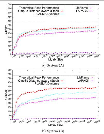
Figure 8. Performance comparisons against existing symmetric matrix inversion implementations
