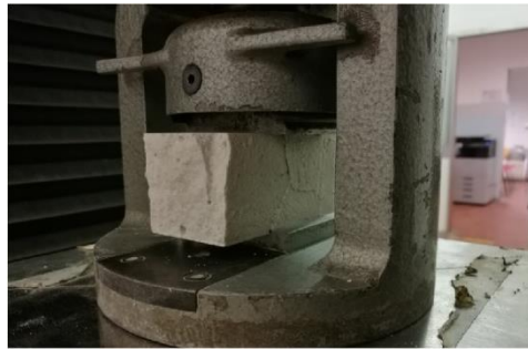
Figure 4: Compressive tests to characterize the bi-component composite material used for the blocks.
