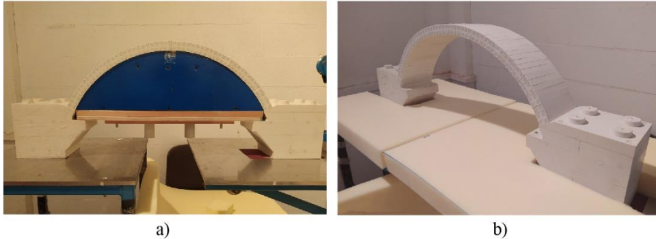
Figure 2: Physical model: a) plywood scaffolding, b) view after the removal of the scaffolding.
