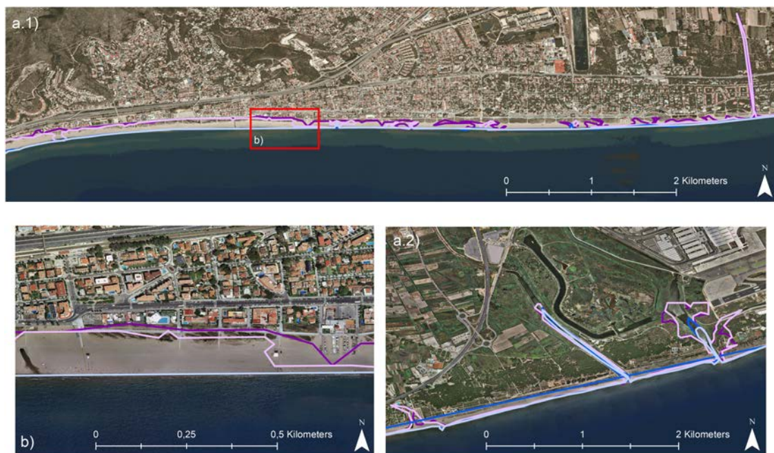
FIGURE 5 Flooding lines distribution of Unit 8. (A.1, A.2) General views of the unit. (B) Close-up view. Light blue = actual conditions, RP = 50 years; dark blue = actual conditions, RP = 500 years; light lilac = RCP8.5, RP = 50 years; and dark lilac = RCP8.5, RP = 500 years.
