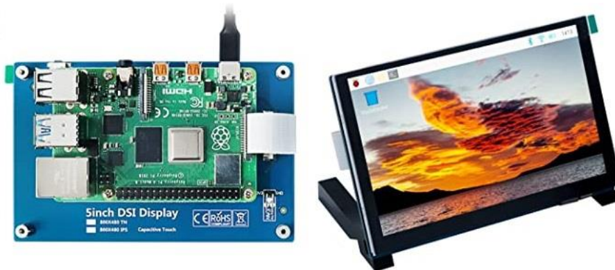
Fig. 4.3: Back (left) and frontal (right) view of the screen. Mounting not used.
