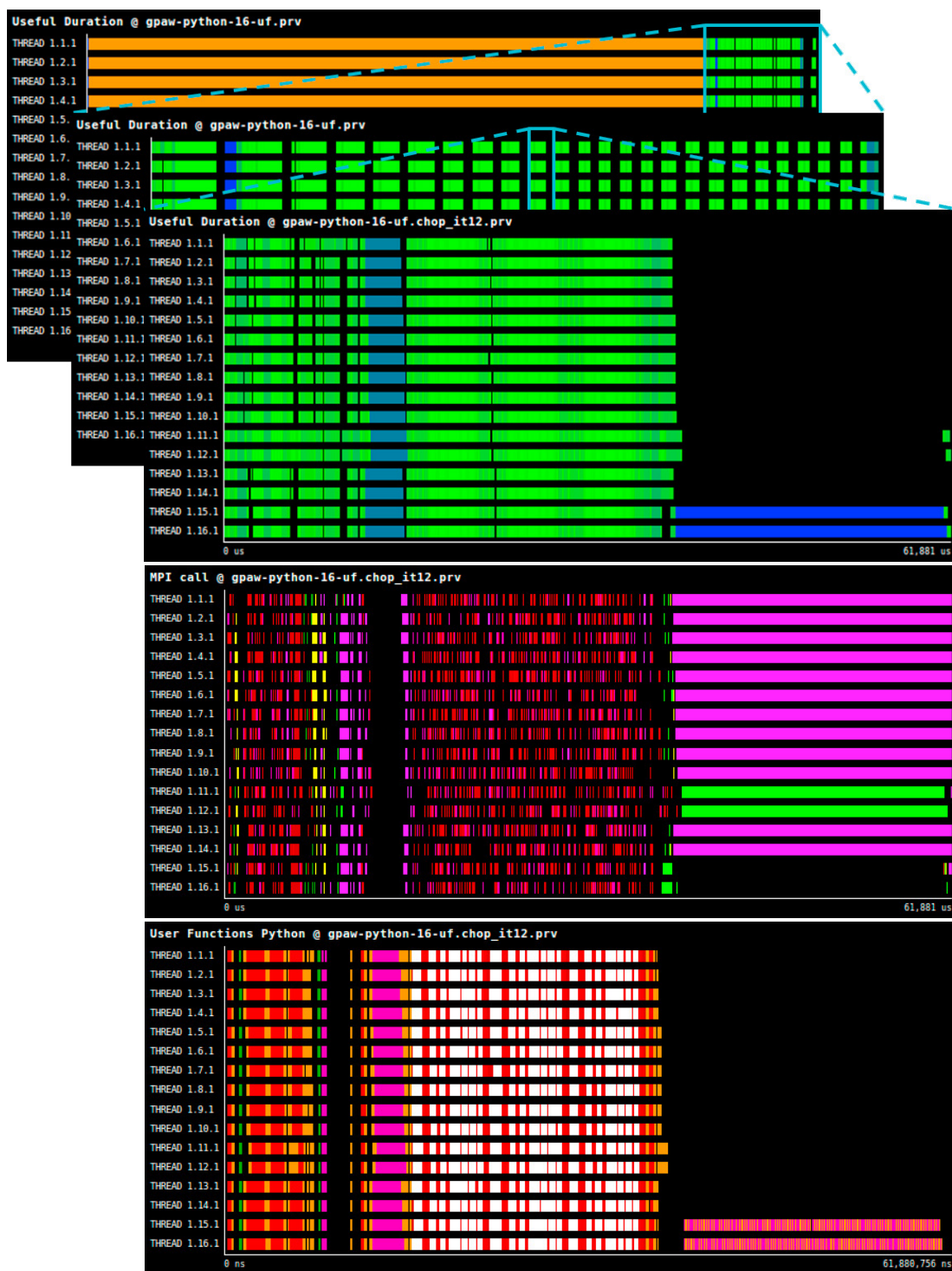
Figure 1: Analysis of the H2 molecule example with Paraver. Top: Useful duration for the entire application (background), a zoom to the iterative phase, and a zoom into the 12th iteration. Center: Display of the MPI activity. Bottom: Timeline of Python user functions.
