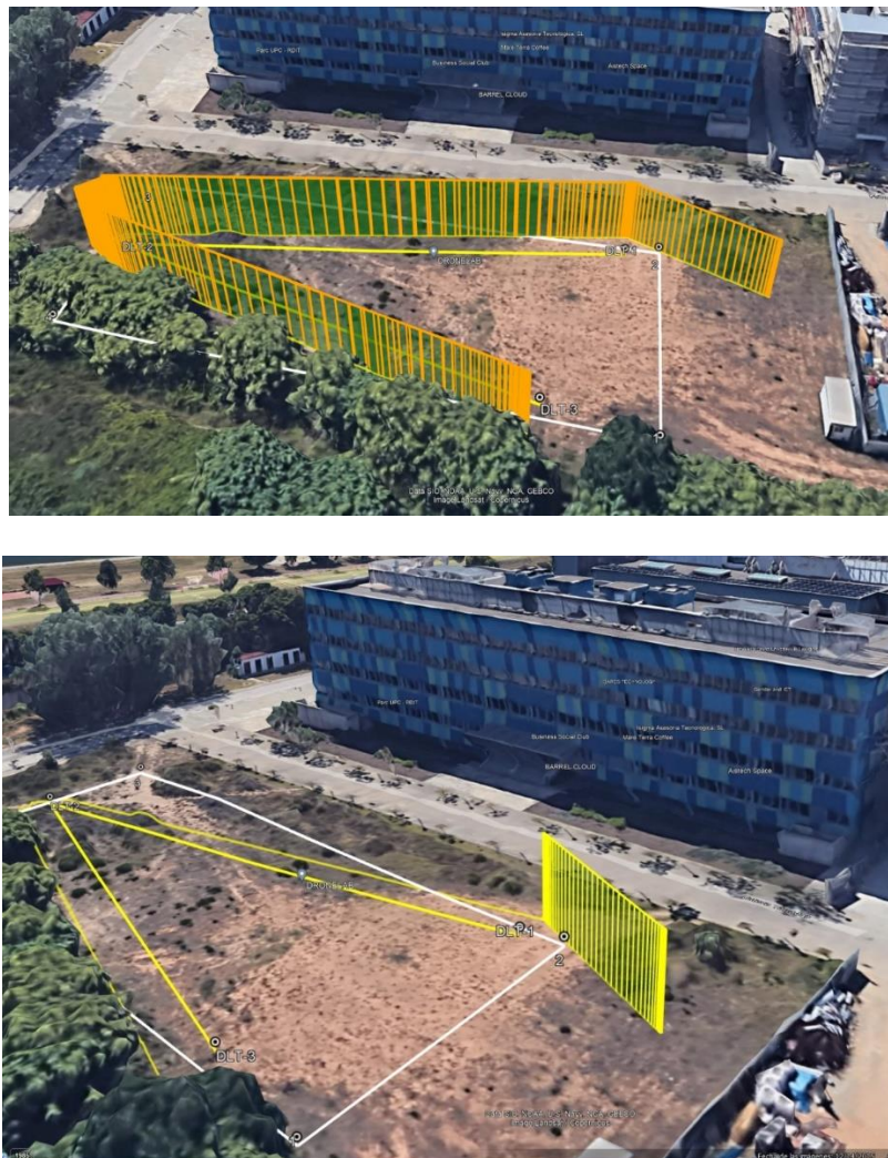
Fig. J.1 Tower inspection flight path (upper) and RTL slope (lower)
