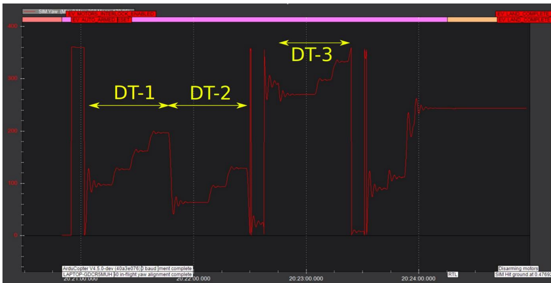
Fig. J.2 Yaw angle increase to scan each tower
