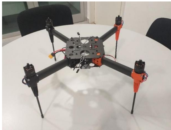
Fig. 2.6 Hexsoon EDU450 kit during its assembly [8]
