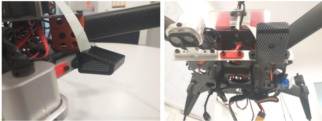
Fig. E.1 Original fixed-position camera mount
