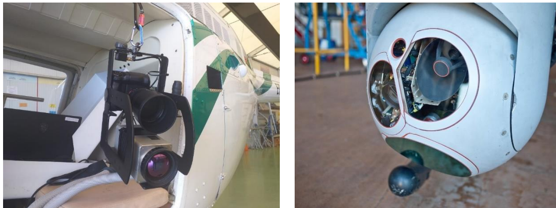
Fig. 2.1 DSLR camera above and thermal camera below (left) and WESCAM MX-15 [27] camera (right).
