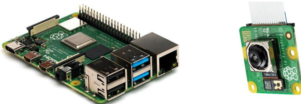
Fig. 2.11 Raspberry Pi board (left) and the RPi V2.1 camera (right)
