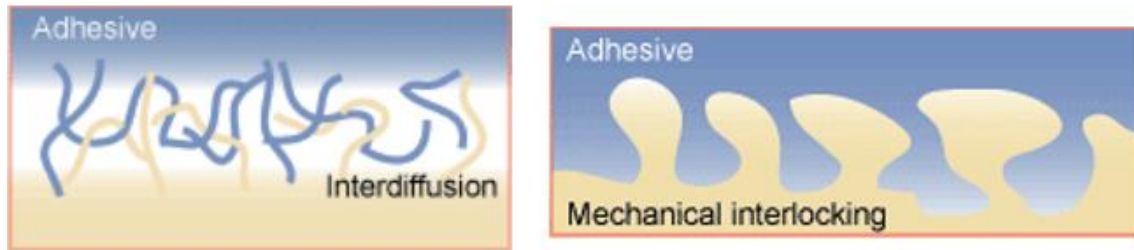
Fig. 1.4 On the left, diffusion or interdiffusion. On the right, mechanical interlocking [19].
