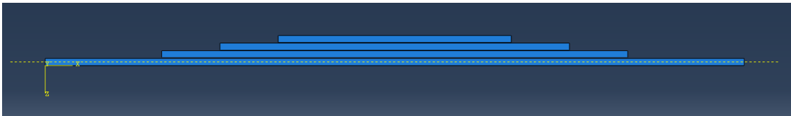
Fig. 5.4 Specimen before forces are applied; dotted line is symmetric plane.
