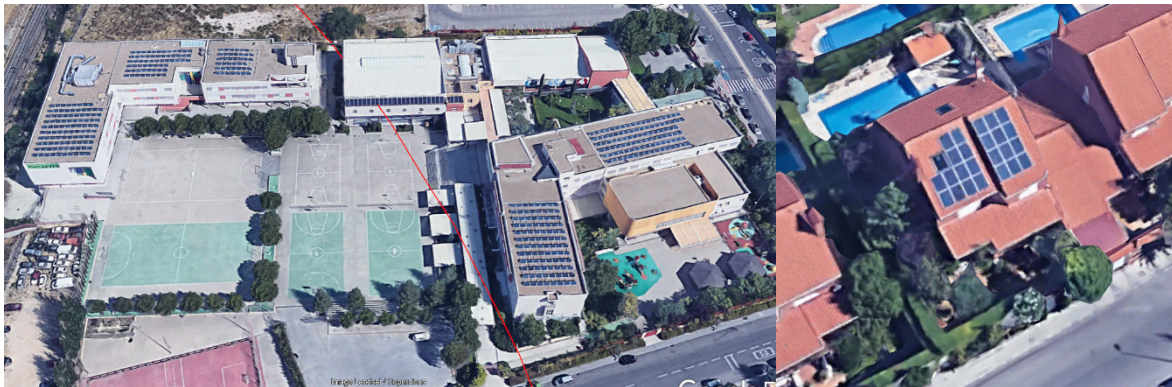
Figure 22. PV panels oriented in the main axis of the building.
