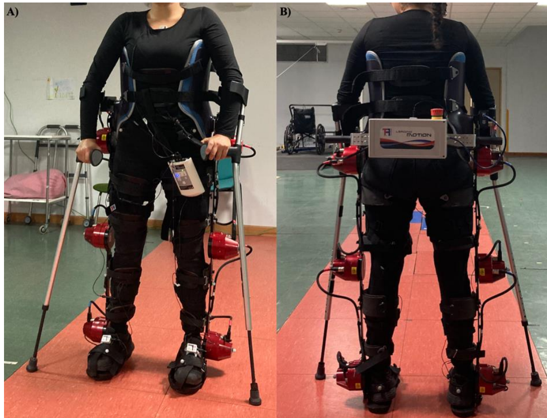
Figure 27. Part II, condition 2: exoskeleton-assisted walking test with Exo-H3, IMUs and Vicon instrumentation. A) Frontal view. B) Back view.
