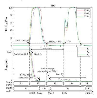
**Figure 11.** MSOGI-THD protection method behavior during a 3PH-G fault with 2DGs at F1. Upper:  $THD_{abc}$ . Lower:  $\widetilde{A}_{abc}$ .
