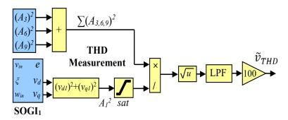
Figure 3. Block diagram of the MSOGI-THD measurement method.
