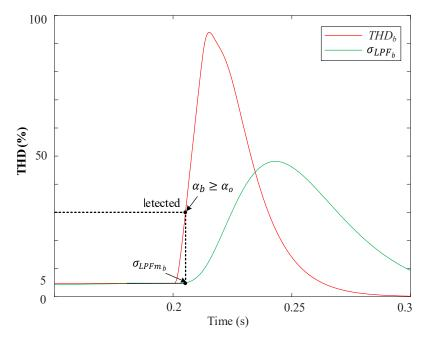
**Figure 8.** An example of the behavior of  $THD_b$  and  $\sigma_{LPF_b}$  during a fault of phase "b" with the proposed fault detection algorithm.
