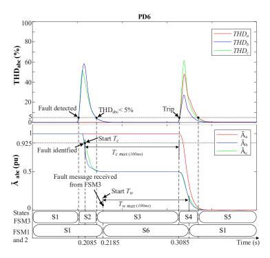
**Figure 14.** MSOGI-THD protection method behavior during a 2PH fault without DGs at F2. Upper:  $THD_{abc}$ . Lower:  $\widetilde{A}_{abc}$ .
