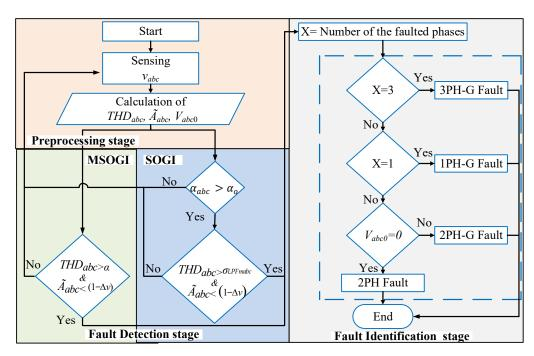
Figure 9. Flowchart of the fault classification algorithm.
