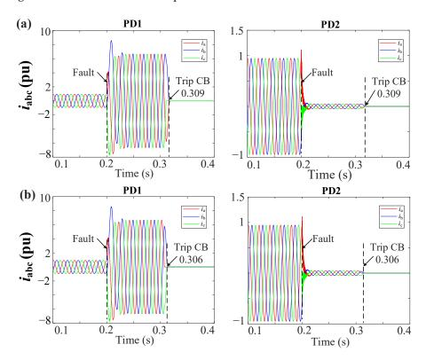
**Figure 13.**  $i_{abc}$  currents for the grid during a 3PH-G fault with 2DGs at DL1 using (a) MSOGI-THD and (b) SOGI-THD.
