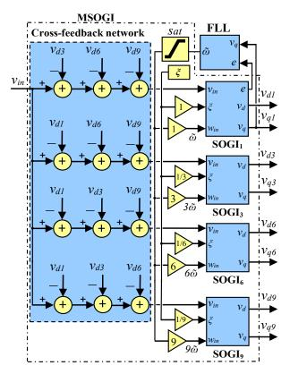
Figure 2. Block diagram of the MSOGI-FLL.
