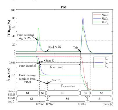
**Figure 15.** SOGI-THD protection method behavior during a 2PH fault without DGs at F2. Upper:  $THD_{abc}$ . Lower:  $\widetilde{A}_{abc}$ .
