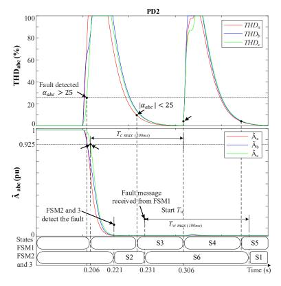
**Figure 12.** SOGI-THD protection method behavior during a 3PH-G fault with 2DGs at F1. Upper:  $THD_{abc}$ . Lower:  $\widetilde{A}_{abc}$ .
