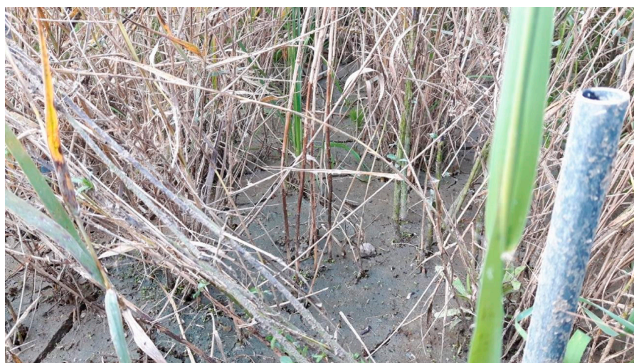
Figure 6. View of the retained digestate layer laying on the bed of the STW. Note the extensive crack on the left-hand bottom of the picture. Images credits: Center for Recirkulering v/Peder Gregersen.
