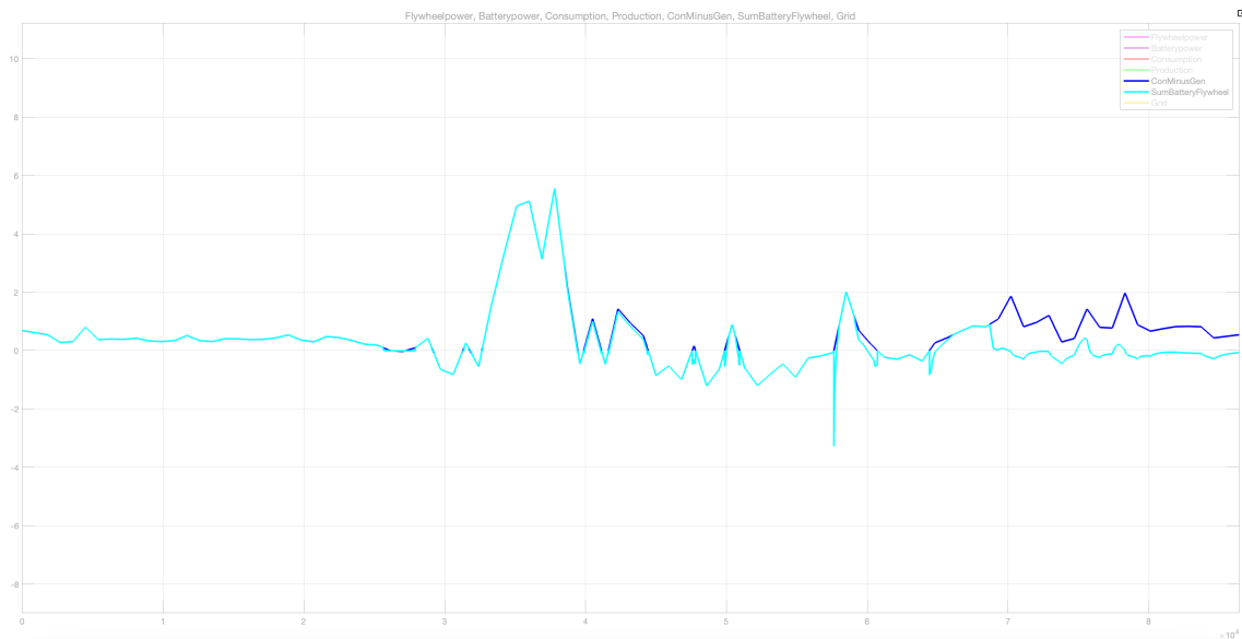
Figure 4.32: Battery power plus flywheel power(cyan)-Consumption minus generation(blue)
