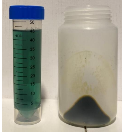
Figure 16. Left container with the supernatant with accumulated pigments and right container with pellet of Synechocystis sp. after centrifugating for 14 min at 7000 rpm.
