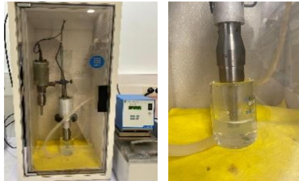
Figure 5 & 6 : 750 Watt ultrasonic processor
