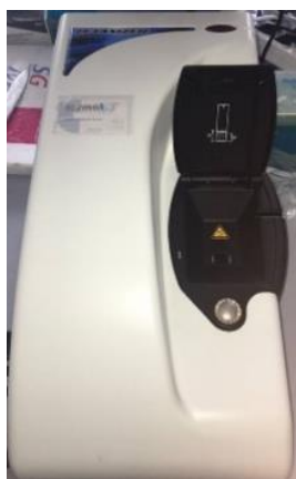
Figure 9 : Zetasizer Nano Z (Malvern Instruments)
