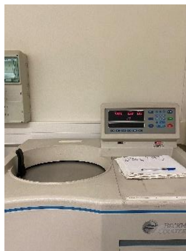
Figure 7 : Ultracentrifuge (Beckman Coulter (Optima LE-80K))
