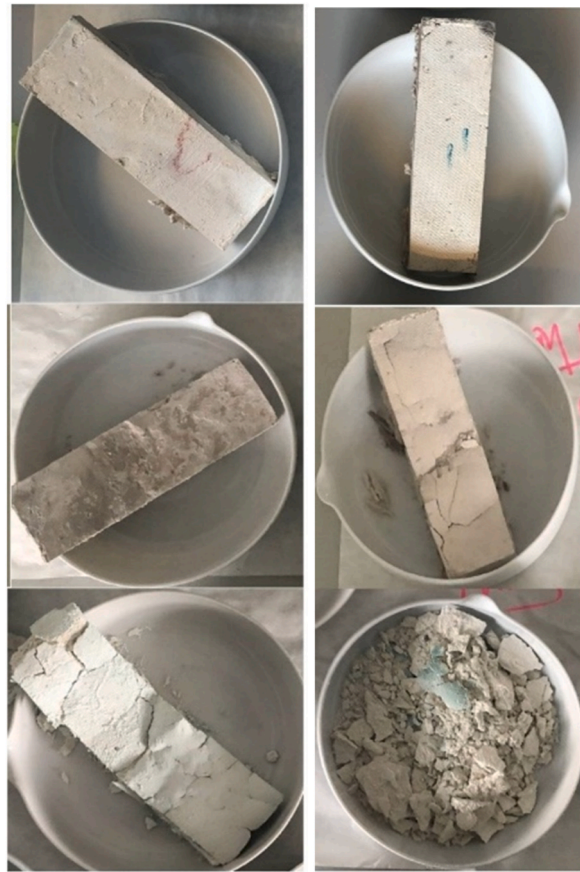
Fig. 8. Images of the composites after the small-scale fire test at different temperatures: a) AC-250, b) AC-450, c) AC-950, d) NC-250, e) NC-450, f) NC-950.
