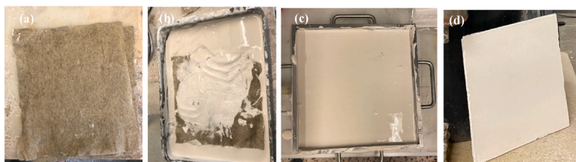
Fig. 2. Lime panel production: a) nonwoven fabric; b) impregnation of the lime paste into the nonwoven fabrics; c) casting in the mold; d) lime boards.
