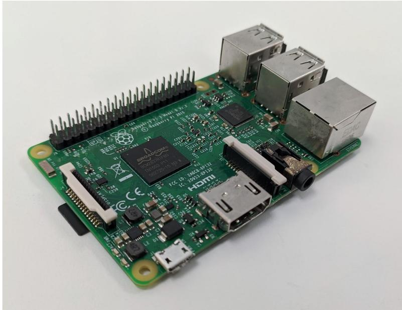
**Figura 1.4.** Raspberry Pi 3 Model B
