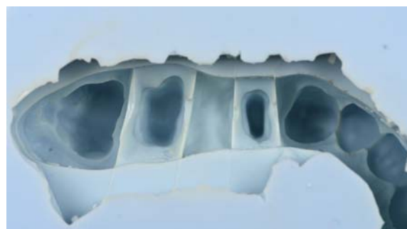
Figure 3. Photographic image of the silicone mold made from the master model.
