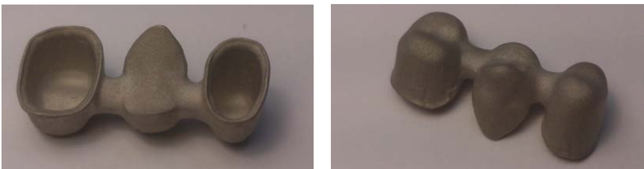
Figure 5. Images of the master model to be reproduced by all the manufacturing centers, with details of its top (left) and bottom (right) views.
