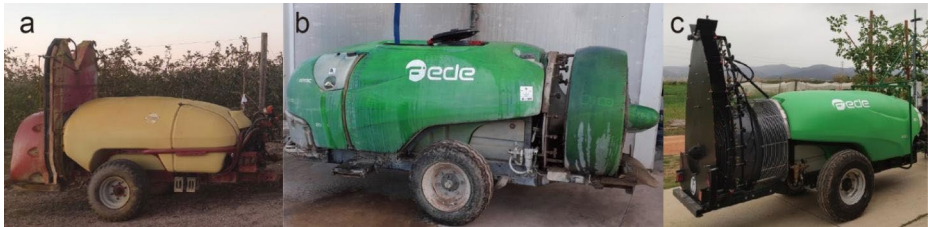
Fig. 1 Three air-assisted spraying systems used for the field trials: a) Hardi tower sprayer, b) Fede axial-fan sprayer, c) Fede tower sprayer.
