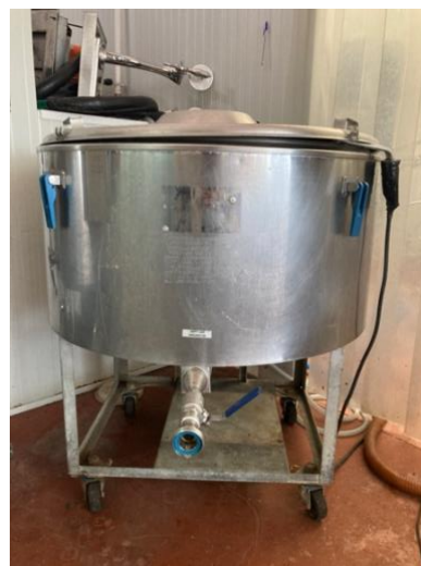
Figure 3.18 & 3.19. Container where the mixture between disinfectant and water is heated up
