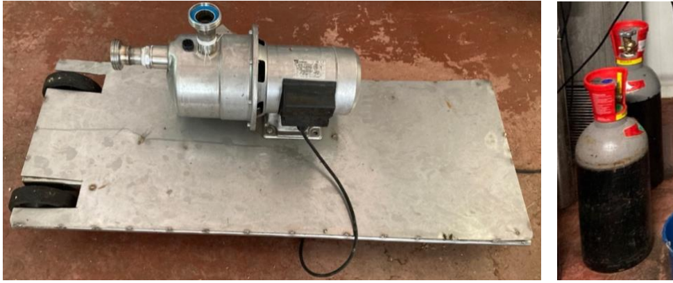
Figure 3.11. Motor used to transfer wort from one container to another
