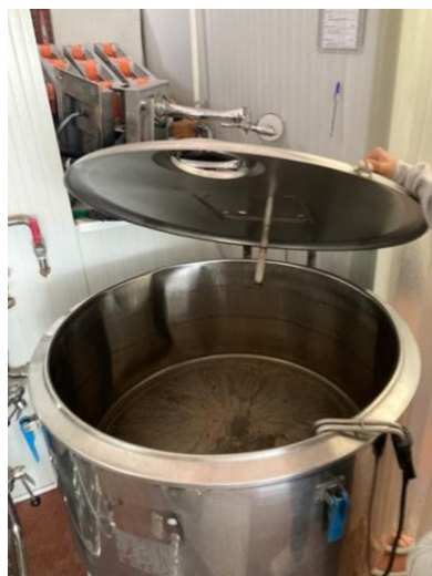
Figure 3.18 & 3.19. Container where the mixture between disinfectant and water is heated up
