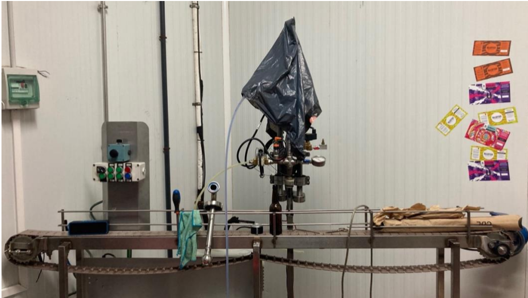
Figure 3.15. Bottling machine used to fill and pack bottles
