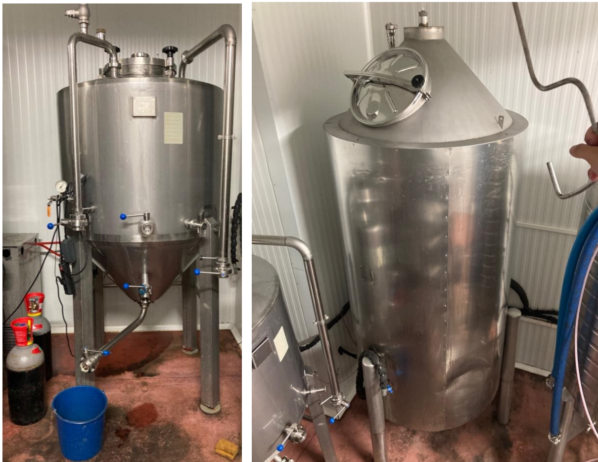
Figure 3.7 & 3.8. Non-adiabatic 1500 litres fermenters (conical on the left and flat on the right)
