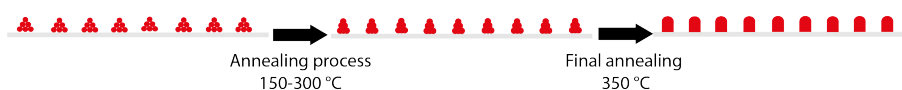
Fig. 2. Steps of the annealing process and how it affects the shape and form of the metamolecules.
